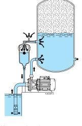
2) When starting, the pumps creates a suction pressure which also takes the water from ARIAMAT, allowing some more water to come from the vessel. The water through the ARIAMAT venturi sucks air from the upper valve.
