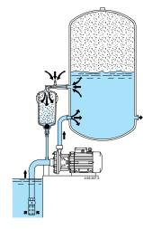
The water level in the ARIAMAT drops until the ball valve moves to the bottom of the ARIAMAT closing the hole of the pipe connected to the pump. ARIAMAT is now full of water.
